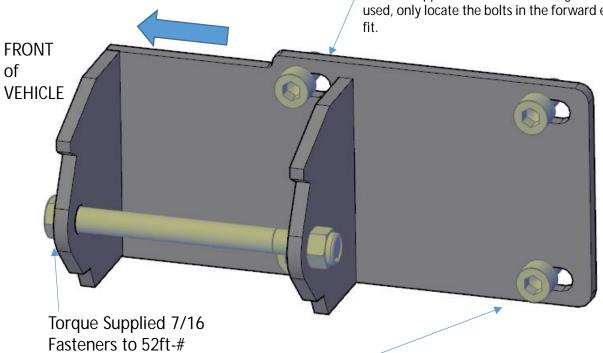
Torque Supplied M10 Fasteners to 36 ft-#
